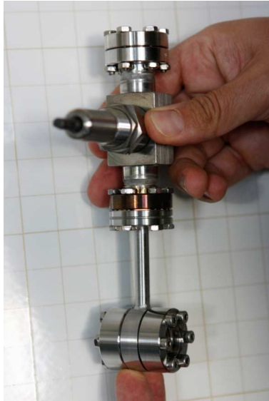
Fig. 2. Optical timing cell, outside of its housing. Two fast photomultipliers are mounted on the glass windows looking at the TMBi volume.
